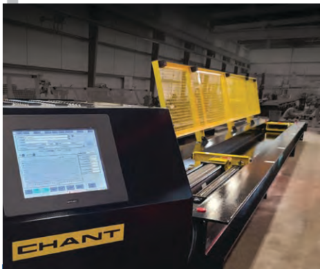
Chant Engineering horizontal test bed with Hydraulic Power Unit.
