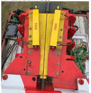
Services, Inc. tested the guy wire to 341,000 pounds. All the testing went well, and the guy wires never left the tower, all completed with much less time and cost than anticipated.
