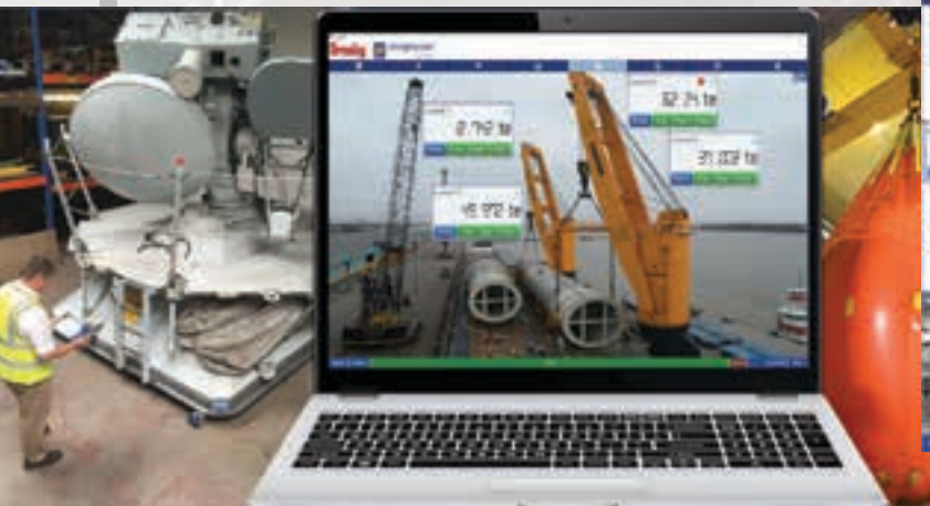
INSIGHT software allows users to monitor up to 126 load cells from up to 700m (2,300 ft.) away.
