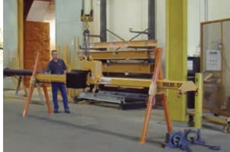
The custom lifting beam is for applications where a crane cannot be positioned over a load due to limited travel or obstructions.
