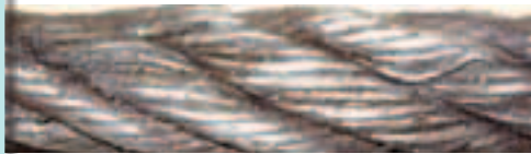
The crushed area of this rope had an approximate 5 percent loss of strength.
