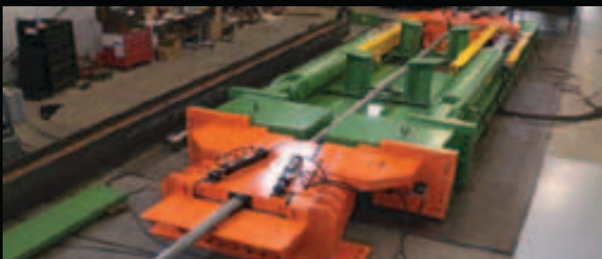
Pre-Stretch Bed with Wire Rope Grips
