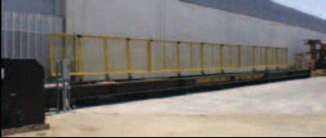
Horizontal Testing Machines 10,000 lbs. to 5,000,000 lbs. capacities - Any Length
