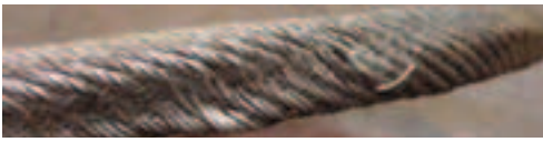
This photo shows crushing that has occurred at a crossover point.
