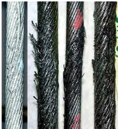
Picture 1: Typical rope damage in multi-layer spooling
