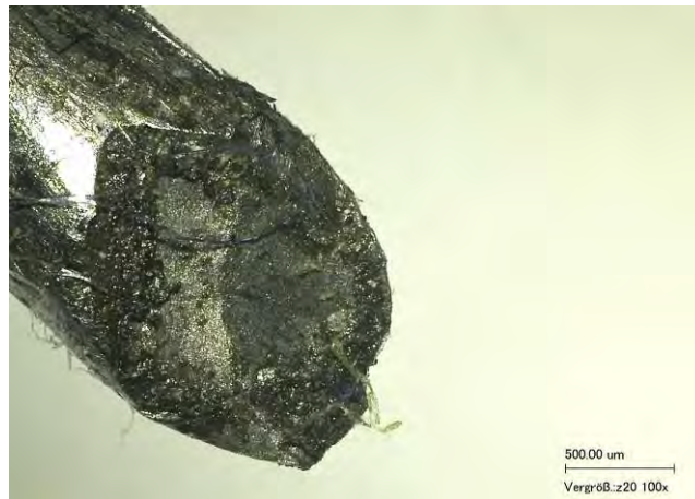
Picture 4: Diagonal wire break
