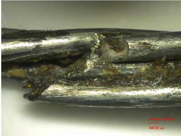
Picture 1: Diagonal wire breaks caused by torsion
