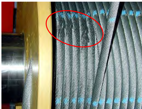
Picture 2: Wire breaks on 1st layer
