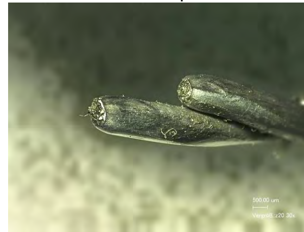
Picture 5: Cup-and-Cone fracture of wires caused by overloading
