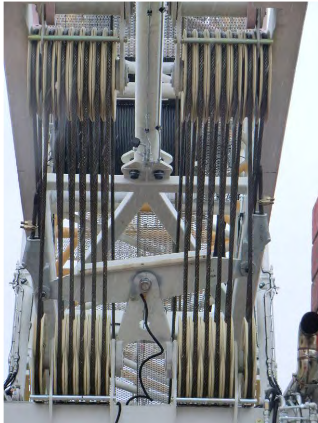
Picture 1: Reeving of an mobile crane
