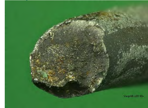
Picture 3: Wire break due to bending of the rope on a sheave
