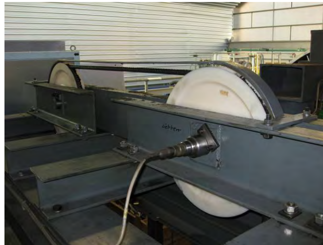
Picture 1: Plastic sheaves used in the multi-layer test stand at IFT
