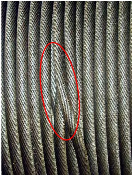
Picture 1: Spooling failure
