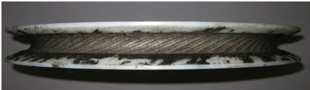
Picture 1: Discarded sheave from the multi-layer test stand at IFT with tooth profile
