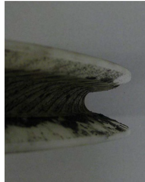
Picture 2: Discarded sheave from the multi-layer test stand at IFT with run in groove
