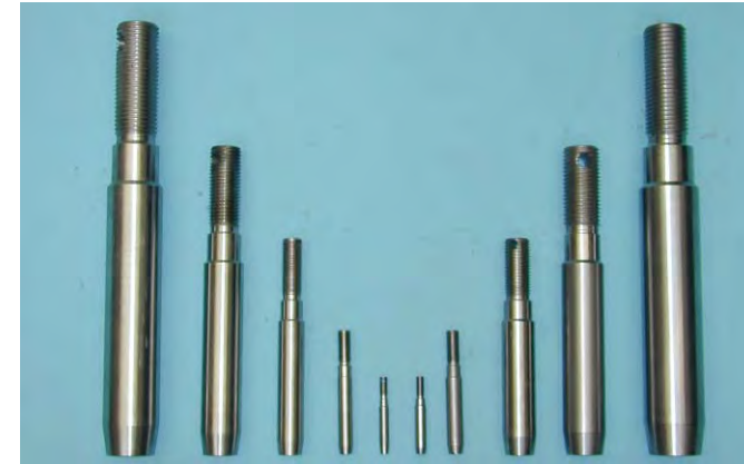
Picture 1: In the research project used swaged external threads
