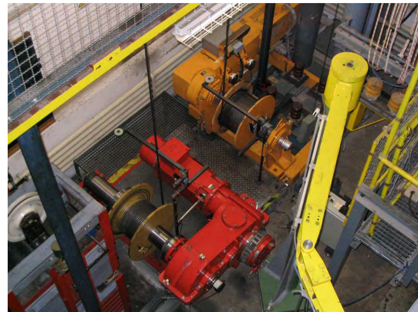
Picture 2: Drums of the multi-layer test stand at IFT, the right drum is the according one to the one displayed in Picture 1
