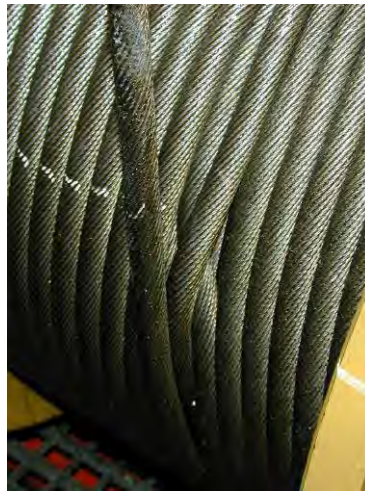
Picture 2 and 3: Spooling failure when spooling with insufficient pretension
