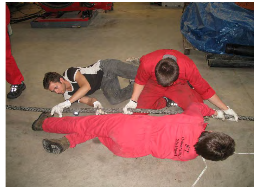
Picture 3: Inspection of a damaged rope at IFT
