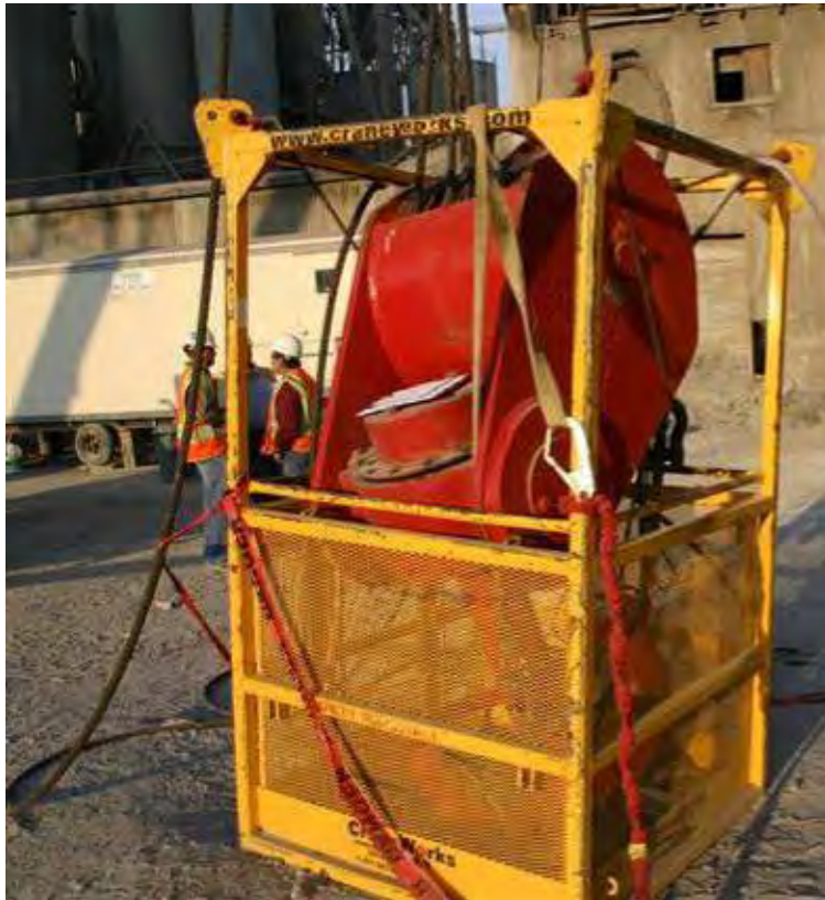
Picture 1: Hook block after rope break
