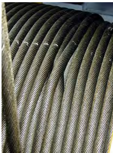
Picture 2 and 3: Spooling failure when spooling with insufficient pretension
