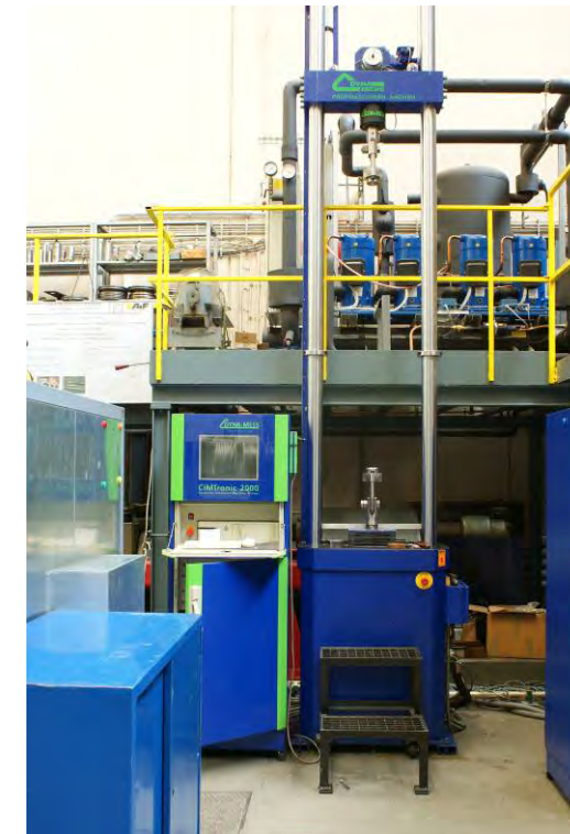
Picture 1: Tension-Tension test machine 75 kN at IFT
