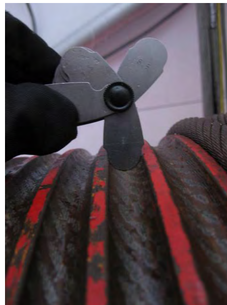
Picture 2: Measurement of the groove radius of a rope drum
