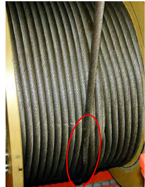
Picture 3: Cutting in of a rope line into the subjacent layer of rope
