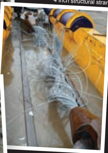
247 tonne load test of a crane boom pendant equalizer link
