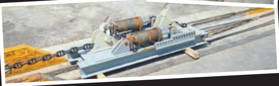
150 ton load test of a custom-built anchor chain jack
