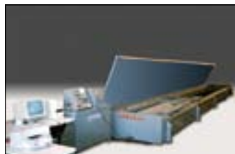
Horizontal Test Bed with Computer system. 150,000 - 3,000,000 lbs.
