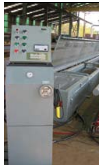
Portable Test Bed (grip available) Capacity: 50,000 - 250,000 lbs.; 20, 30 or 40 foot length.
