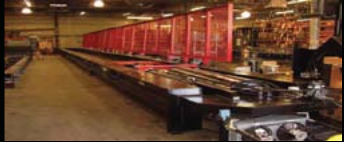
Horizontal Testing Machines 10,000 lbs. to 5,000,000 lbs. capacities - Any Length
