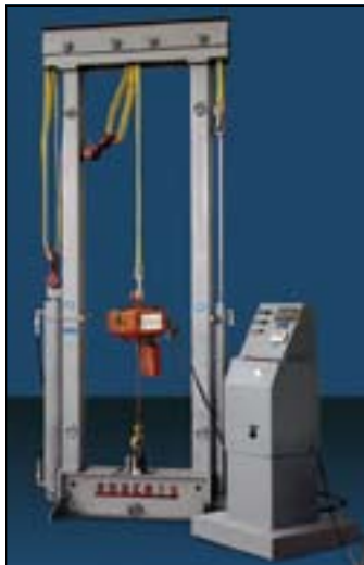
Vertical Test Stand. 50,000 lb. Dynamic testing (hoist moving) or static testing (hoist not moving).
