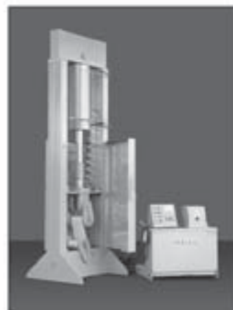
Vertical Break Test Machine. Capacity: 350,000 lbs. with 12" Web Grip.
