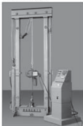
Vertical Test Stand. 50,000 lb. Dynamic testing (hoist moving) or static testing (hoist not moving).
