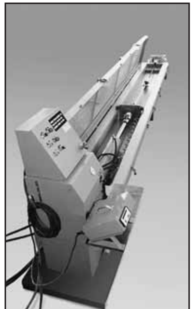
Portable Test Bed with Grip. Capacity: 100,000 lb. - 150,000 lb.; 20, 30 or 40 foot length.
